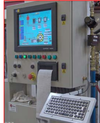
Pictures show typical 15" TFT Colour Screen Display Model with keyboard and thermal printer option
